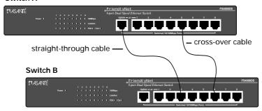
Figure 2-11 Connecting the Switch to another switch or network device
